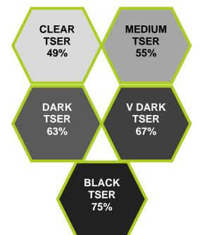
\*TSER indicated for highest performing film in package. TSER for entire package around the full vehicle will be slightly less.
